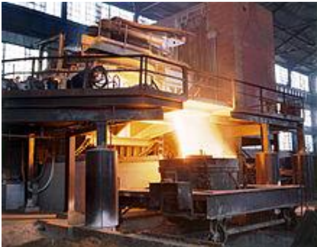
Fig. 8: An arc furnace pouring out steel into a small ladle car. The transformer vault can be seen at the right side of the picture. For scale, note the operator standing on the
